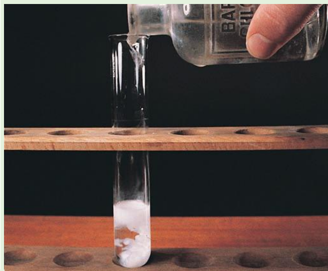
Figure 8.16 When barium chloride solution is added to sodium sulfate a white precipitate of barium sulfate forms.
