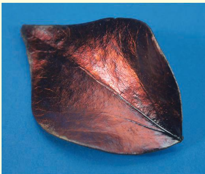
Figure 5.22 This leaf has been electroplated.
