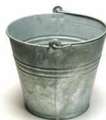
d This bucket has been coated with zinc to prevent the steel of the bucket corroding.
