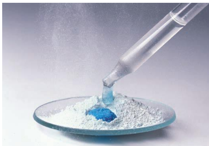
a Anhydrous copper(II) sulfate goes blue when water is added to it.
