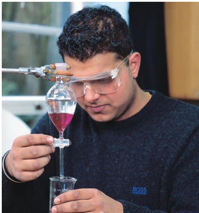
Figure 2.21 The pink liquid is more dense than the clear oil and so sinks to the bottom of the separating funnel. When the tap is opened the pink liquid can be run off.
