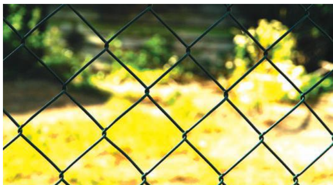
Figure 10.23 A coating of plastic stops metal objects coming into contact with oxygen or water.
