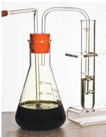
Figure 9.13 Iodine being displaced from potassium iodide solution as chlorine is bubbled through.
