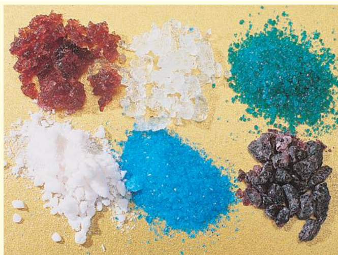
Figure 8.20 Hydrate crystals (left to right): cobalt nitrate, calcium nitrate and nickel sulfate (top) and manganese sulfate, copper sulfate and chromium potassium sulfate (bottom).
