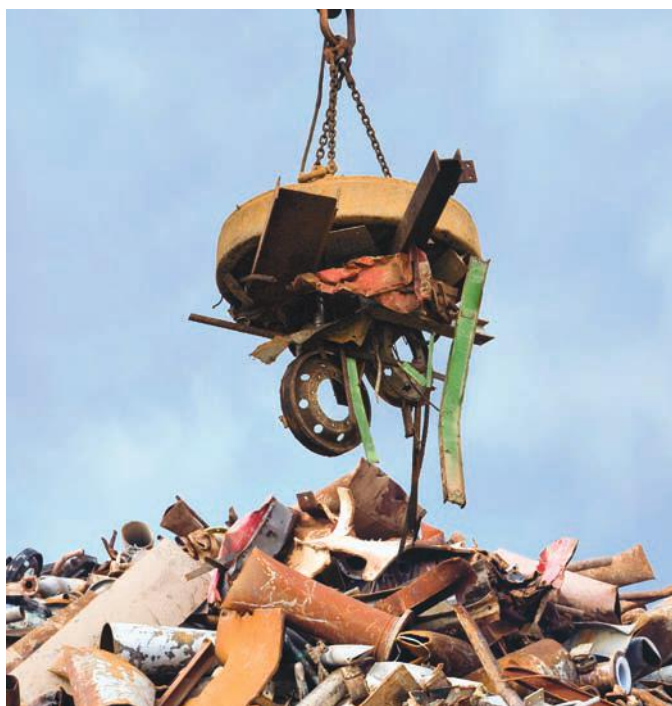
Figure 2.24 Magnetic separation of iron-containing materials.
