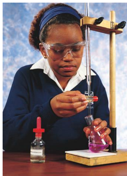
Figure 8.13 The acid is added to the alkali until the indicator just changes colour.
