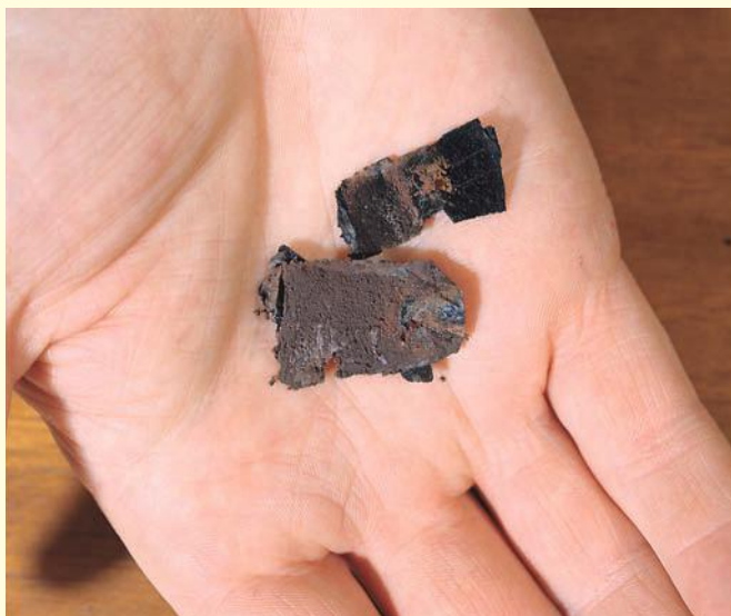
Figure 5.21 This plastic has been coated with copper by electrolysis.
