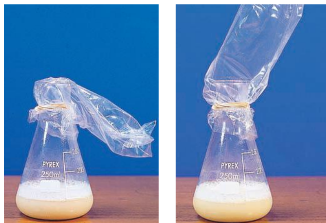
Figure 15.8 Fermenting glucose and yeast to produce ethanol. The bag is inflated during the experiment by CO 2 .
