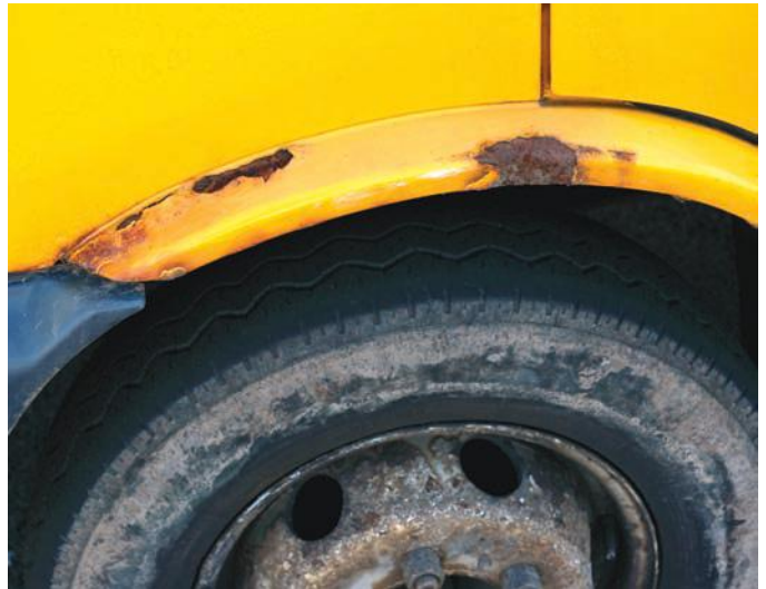
Figure 10.22 A brand new car is protected against corrosion (top). However, if the paintwork is damaged, then rusting will result.
