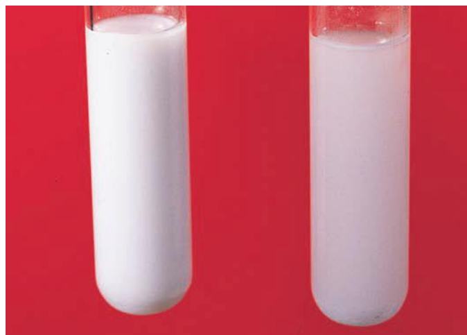
Figure 8.18 If left to stand the white precipitate of silver chloride goes grey. This photochemical change plays an essential part in black and white photography.
