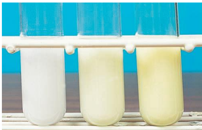
Figure 8.19 AgCl, a white precipitate, AgBr, a cream precipitate, and AgI, a yellow precipitate.
