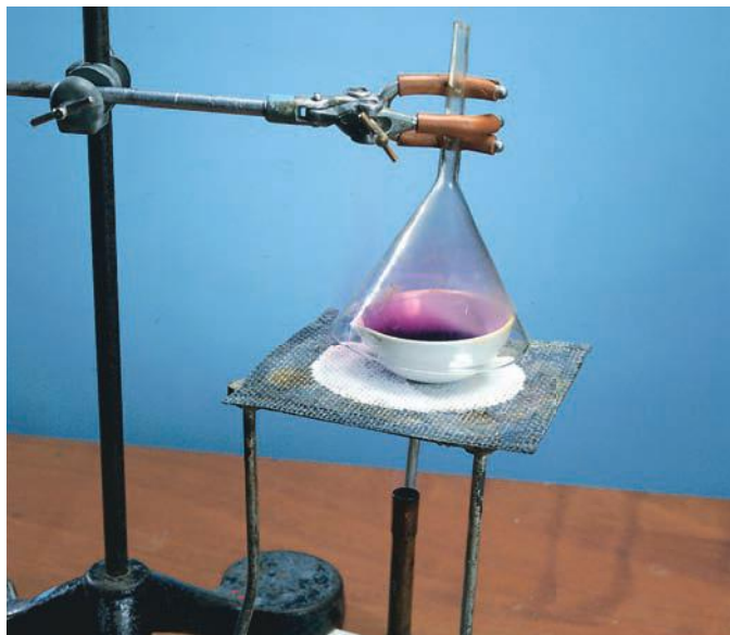
Figure 2.25 Apparatus used to separate an iodine/salt mixture. The iodine sublimes on heating.
