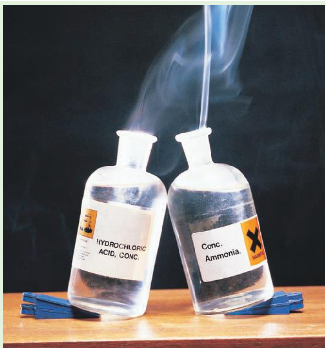
Figure 8.8 The hydrogen chloride molecule (from concentrated hydrochloric acid) acts as a hydrogen ion donor. The ammonia molecule (from concentrated ammonia) acts as a hydrogen ion acceptor.
