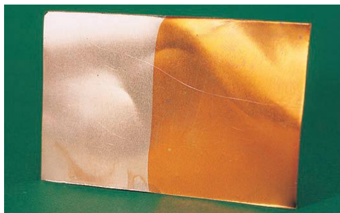
Figure 8.14 Citric acid has been used on the right-hand side of this piece of copper metal to remove the oxide coating on its surface, giving it a shinier appearance.
