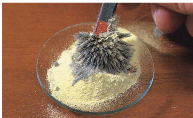
Figure 2.12 A magnet will separate the iron from the mixture.
