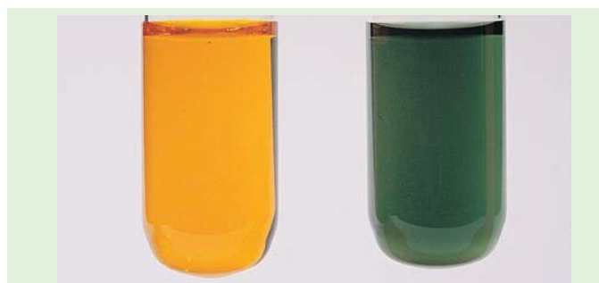
Figure 15.5 Orange potassium dichromate(VI) slowly turns green as it oxidises ethanol to ethanoic acid. Potassium manganate(VII) turns from purple to colourless.
