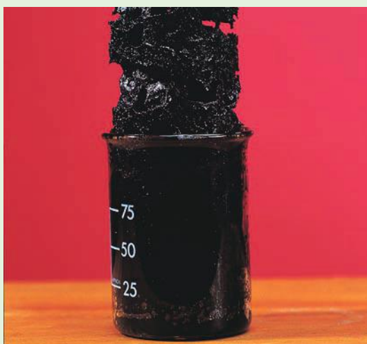
Figure 12.9 The concentrated sulfuric acid has removed the elements of water from the sugar, leaving black carbon.
