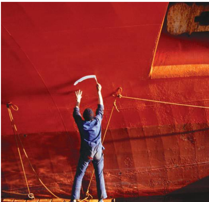
Figure 10.21 Painting keeps the air and water away from the steel used to build a ship.
