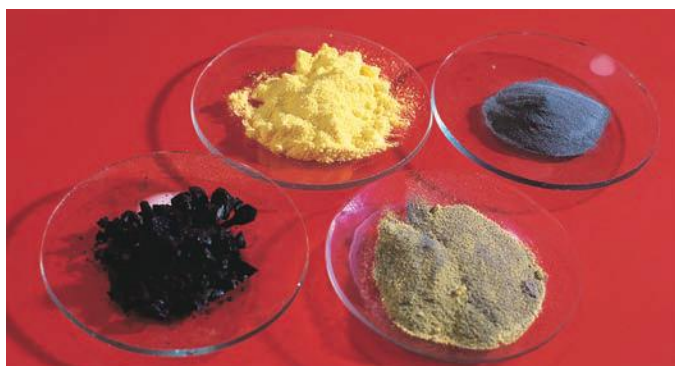
Figure 2.11 The elements sulfur and iron at the top of the photograph, and (below) black iron(II) sulfide on the left and a mixture of the two elements on the right.
