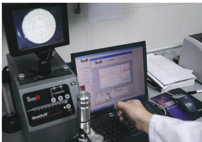
Figure 2.9 This is a modern infrared spectrometer. It is used in analysis to obtain a so-called fingerprint spectrum of a substance that will allow the substance to be identified.
