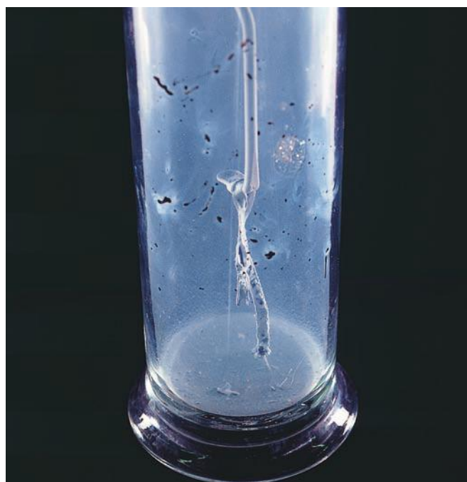
Figure 13.17 When magnesium burns in carbon dioxide gas, magnesium oxide (white) and carbon (black) are produced.
