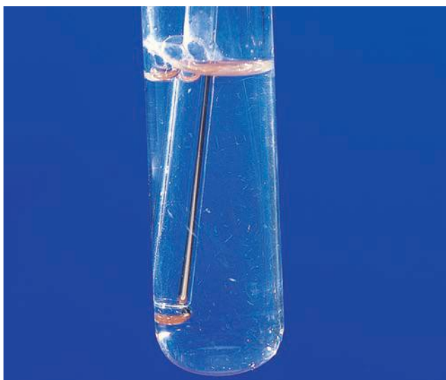
c If the \text{CO}_2 is bubbled for longer the white precipitate dissolves. Figure 13.10 Testing for carbon dioxide.
