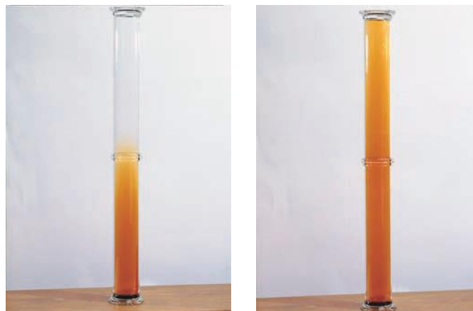
Figure 1.13 After 24 hours the bromine fumes have diffused throughout both gas jars.
