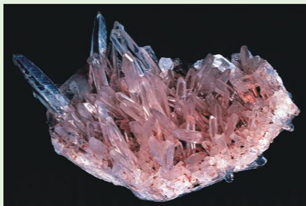
b Quartz is a hard solid at room temperature. It has a melting point of 1610 °C and a boiling point of 2230 °C.
