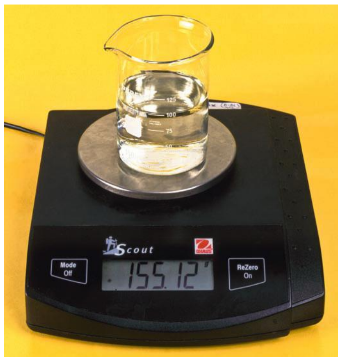
Figure 2.33 An electronic balance can be used to measure the mass of reagents.
