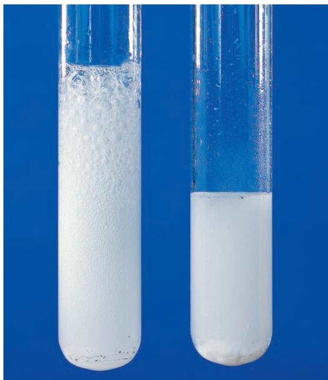
Figure 7.3 The powdered limestone (left) reacts faster with the acid than the limestone in the form of lumps.
