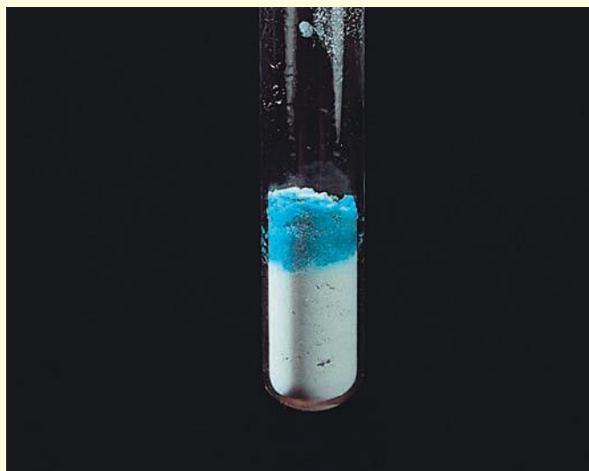
Figure 8.21 Anhydrous copper(II) sulfate is a white powder which turns blue when water is added to it.
