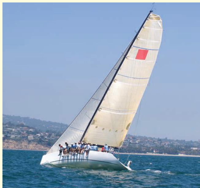
Figure 2.41 The glass-reinforced plastic used to make boats like this is a composite material.
